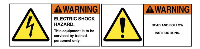
The lightning flash with the arrowhead symbol, within an equilateral triangle, is to alert the user to the presence of non insulated dangerous voltage within the products enclosure that may be of sufficient magnitude to constitute a risk of electric shock to humans.
