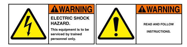
The lightning flash with the arrowhead symbol, within an equilateral triangle, is to alert the user to the presence of non insulated dangerous voltage within the products enclosure that may be of sufficient magnitude to constitute a risk of electric shock to humans.
